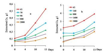
**Fig.1**. Effect of particle size on bioleaching of copper by "Kashen" consortium from sulfide (a) and oxidized (b) ores of Kajaran deposit (PD – 20%, pH –1.8; t – 35<sup>o</sup>C, 180 rpm)
