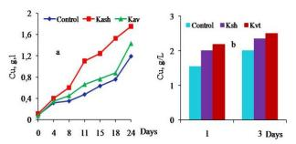
Fig.3. Bioleaching of copper from sulfide (a) and oxidized (b) ore samples by adapted consortia "Kashen" and "Kavart" (PD-20 %, t - 30 °C, 160 rpm)
